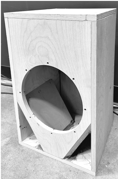
Figure 16. Straight wooden vent installed on Wooden Cabinet prototype
