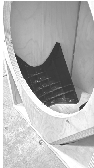
Figure 14. 3D printed flared vent installed on Wooden Cabinet prototype
