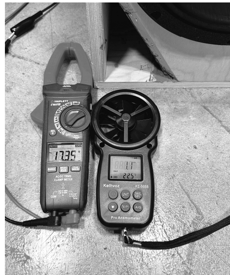
Figure 18. Voltmeter (left) and Anemometer (right) used for measuring Voltage and Air velocity
