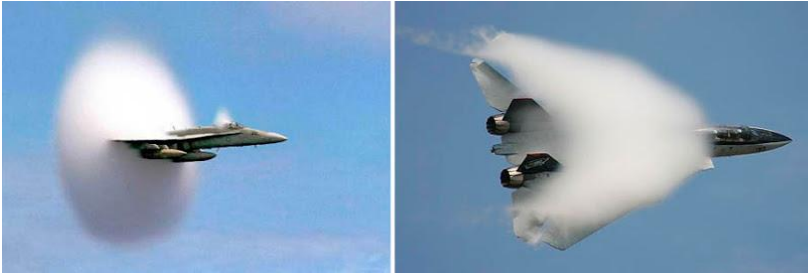
Shock wave formed on supersonic flight (Courtesy:Ensign John Gay, US Navy )
