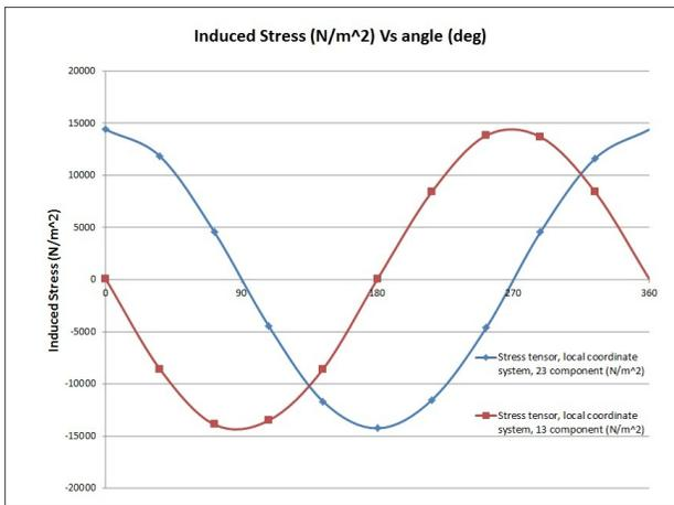
**Figure 2:** Flow direction dependence of induced stress.
