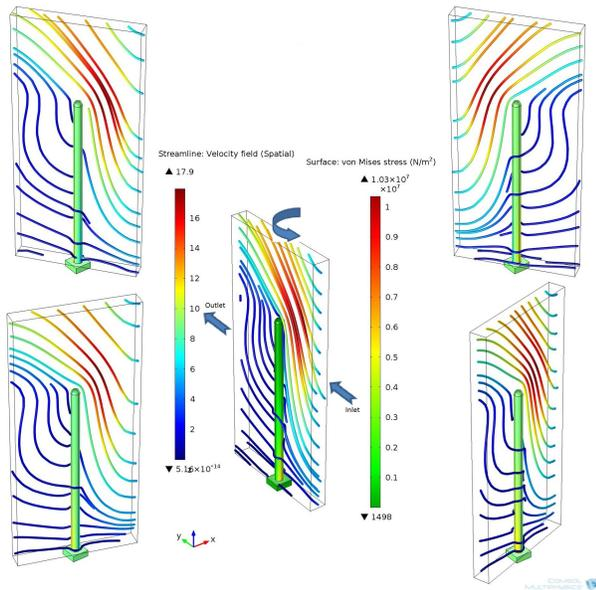
**Figure 1:** Single nanowire model with changing gas flow direction.
