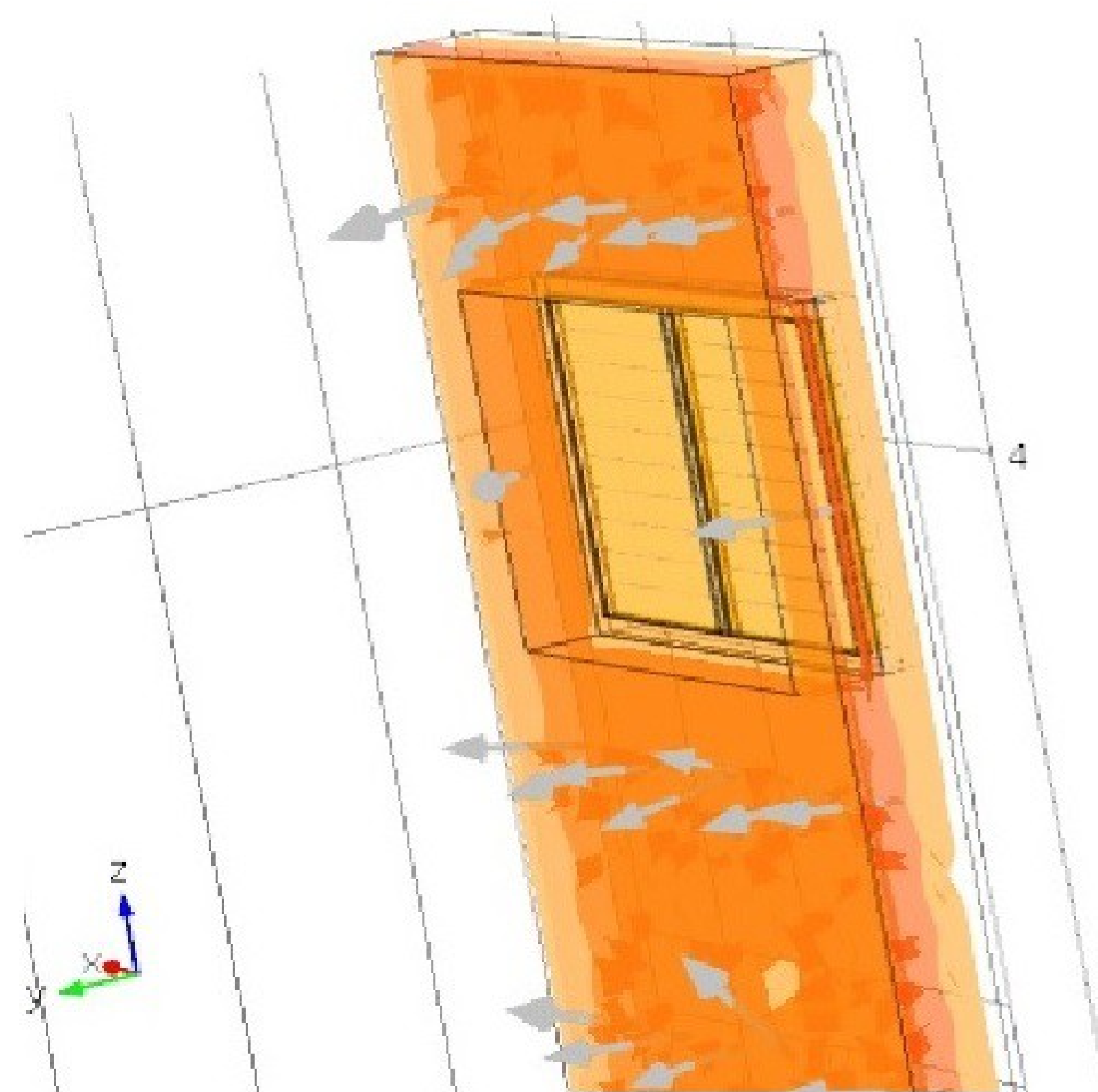
Figure 2. Geometry and plot of iso-thermal contours through the construction
