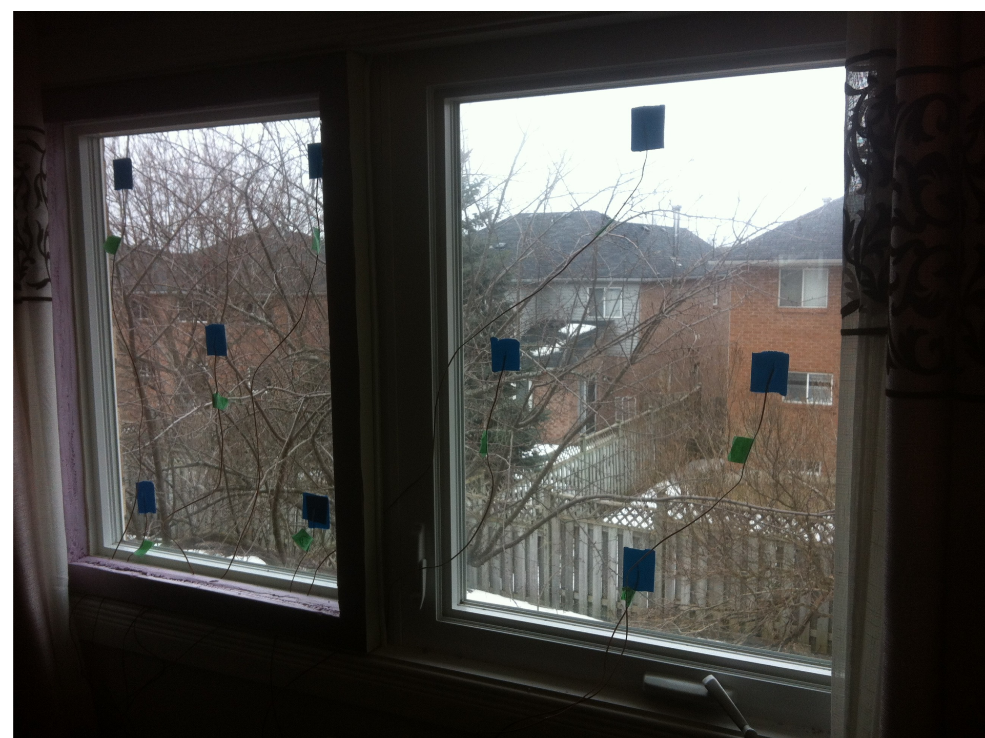
Figure 1. Experimental setup with a static operable insulation system and thermocouples
