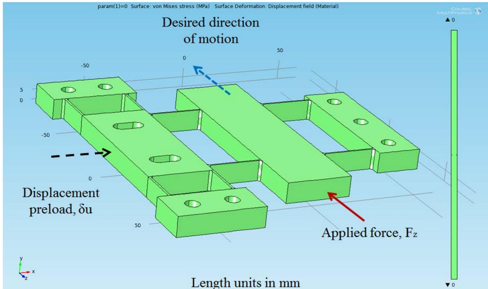
Preload displacement and applied force can be varied without re-meshing
