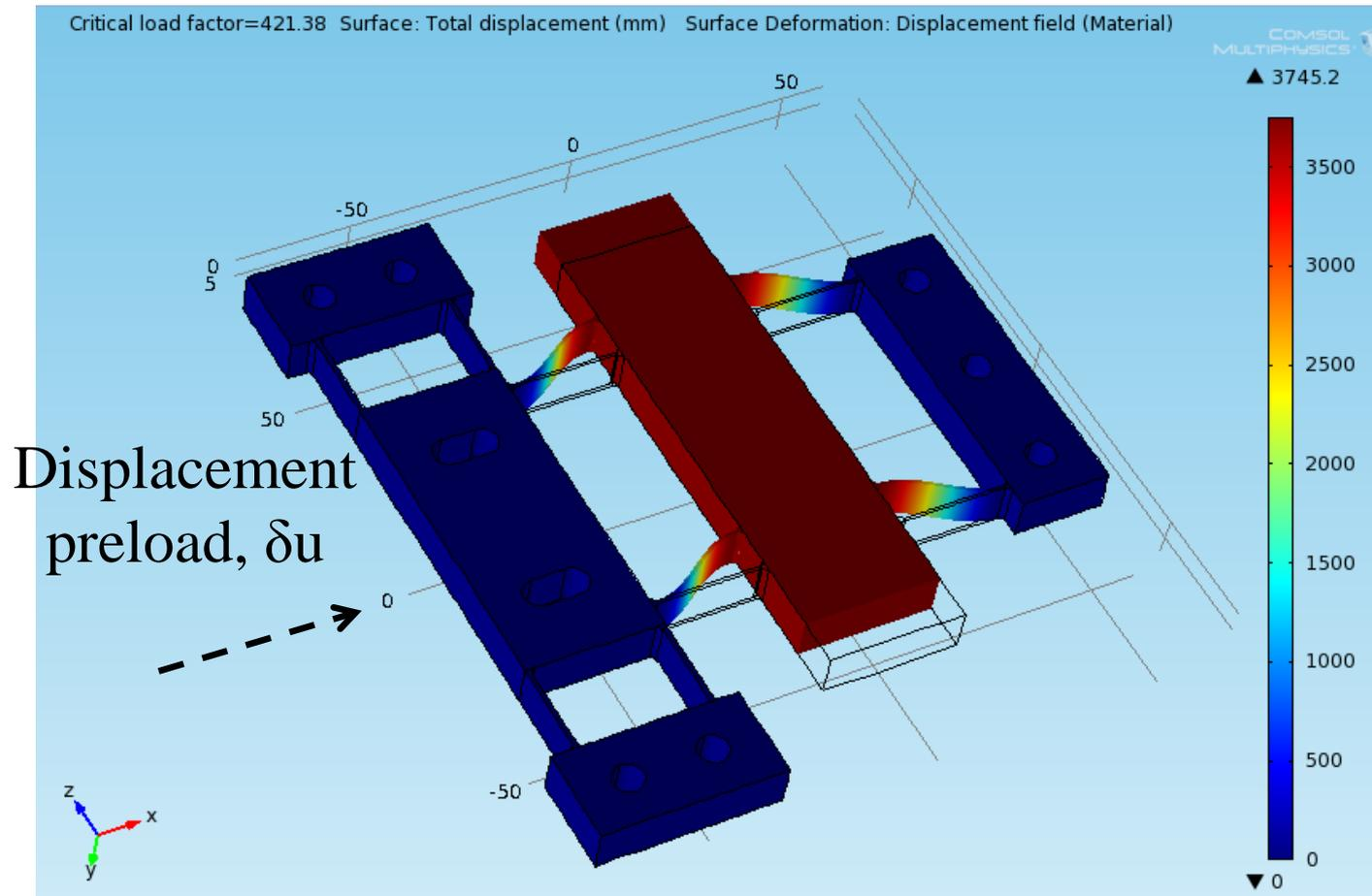
Imperfection shape is obtained from linear buckling analysis
