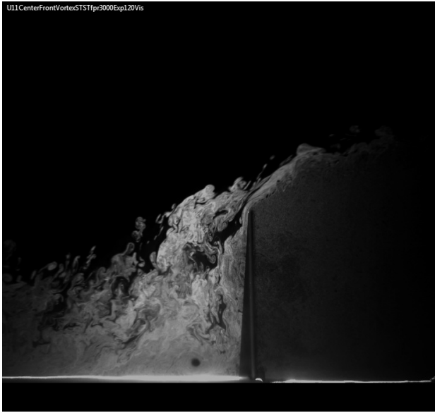
Figure 2: Flow visualization of upstream vortex.
