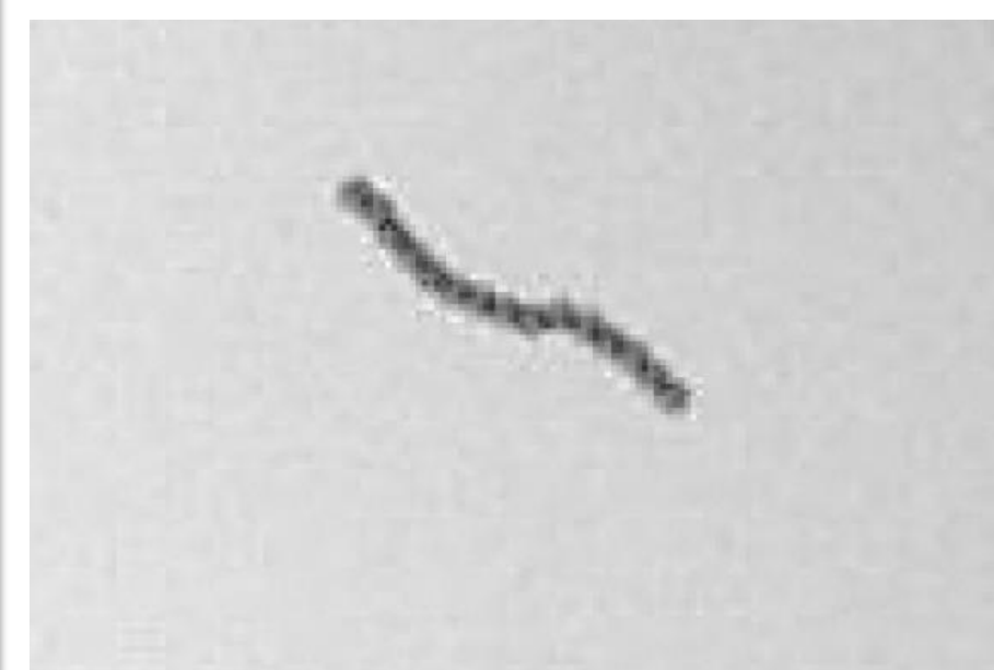
Figure 3c Chain breaking apart as it is not able to follow the rotation of the magnetic field.
