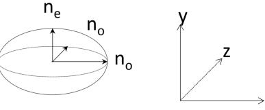
5%MgO:LiNbO<sub>3</sub> is negative uniaxial crystal ( $n_e <$ n<sub>o</sub>), z-cut wafer, with the diameters of up to 4"
