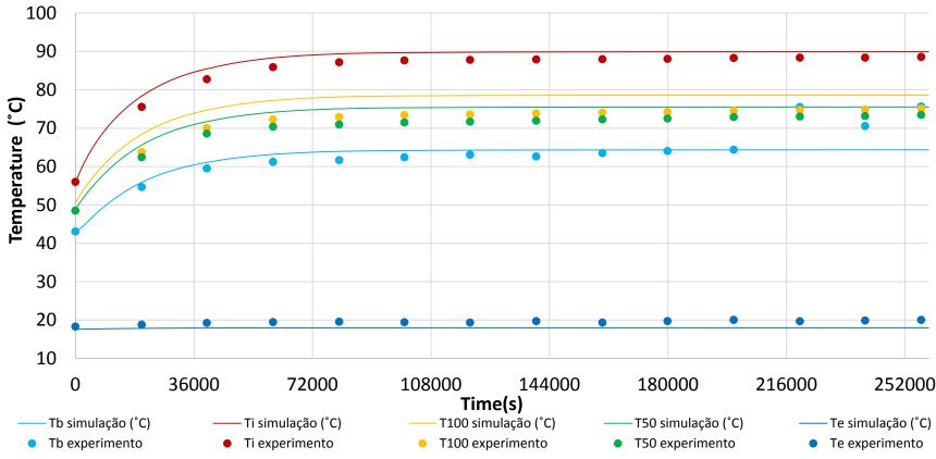
The numerical results obtained for the improved model showed good agreement with experimental values, particularly regarding to  $T_i$  and  $T_b$  temperatures. Therefore, it allows to validate the thermomechanical modeling proposed in this work and the stationary state obtained in both structures.
