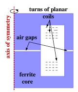
2D axis symmetry model - geometry
