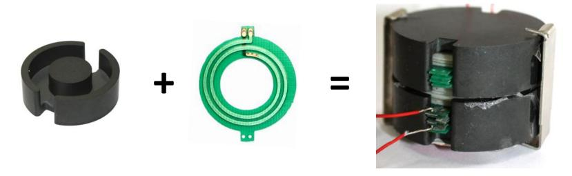
View of the prototype of the multilayer planar transformer and its components: a pot core and a planar coil
