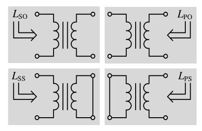
Windings' configurations for the impedance measurements.
