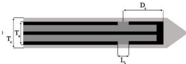
Fig.1 (a) coaxial antenna design
