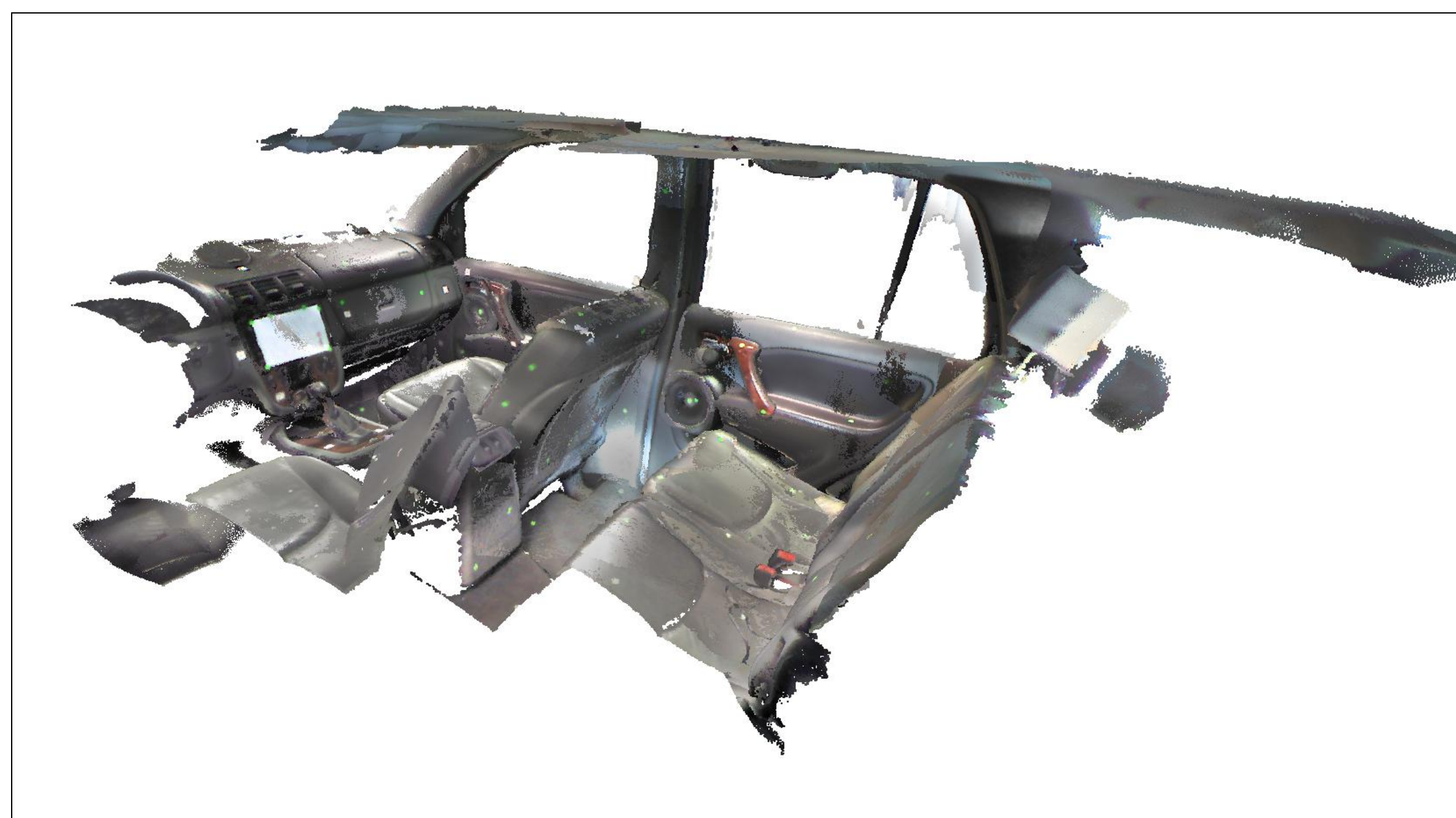
Figure 2. 3D scan of the car cabin
