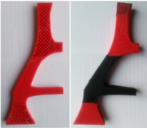
Figure 3: 3d printed optimized part with heterogeneous infill (left) and multimaterials (right)
