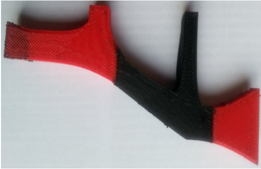
Figure 5. - Optimized structure printed with two different materials
