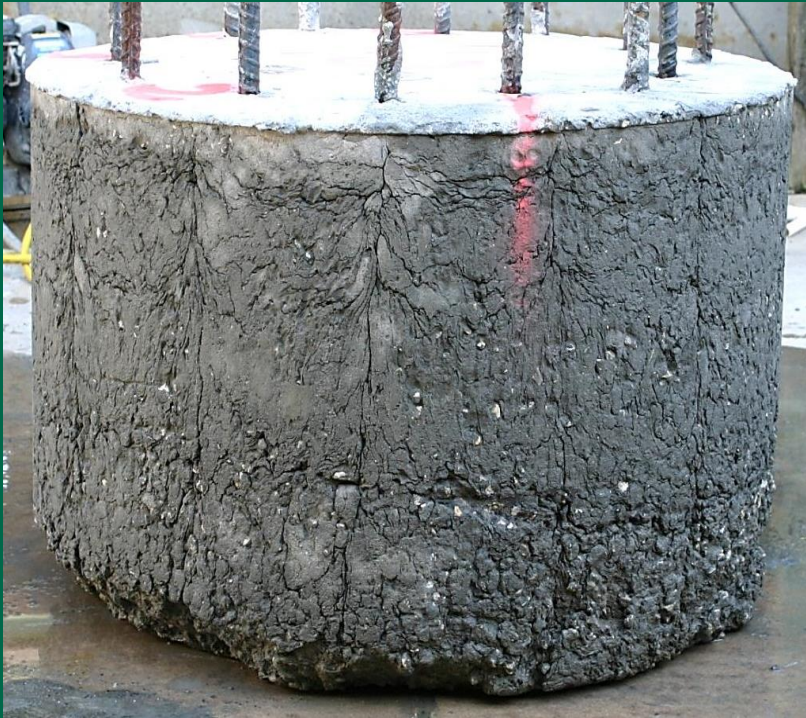
cast under mineral slurry, 40 sec/qt.
