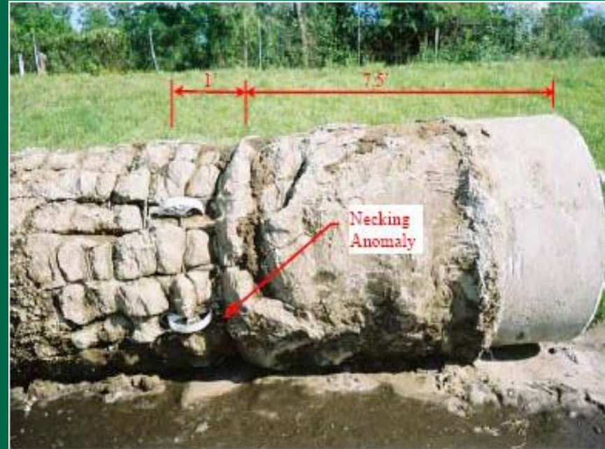
Shaft exhumed -poor concrete flow performance
