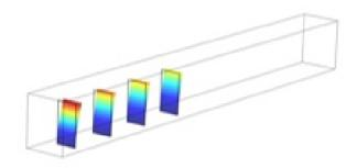
**Figure 1**: Displacement of Piezoelectric Plates inside of a Quarter-Wavelength Straight Tube Resonator
