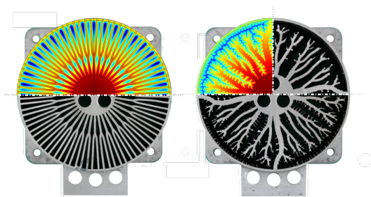
Figure 7. Simulation results and prototypes. Parametric optimum: top - simulation, bottom - printed and post processed part. Topological optimum: upper left - simulation, upper right - printed and post processed part without forced edging. bottom - printed and post processed part with forced edging.
