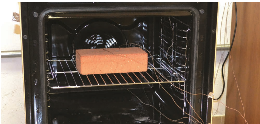
FIGURE 1: Whirlpool's Minerva oven set up for the "brick test."
