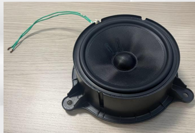
Cone: Fiberglass Surround: Nitril Rubber 60A
