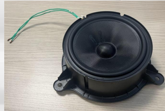
Cone: Fiberglass Surround: Nitril Rubber 60A
