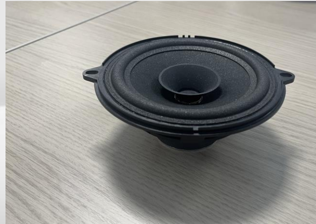
Cone: Paper +10% Mica Surround: Polyurethane Foam
