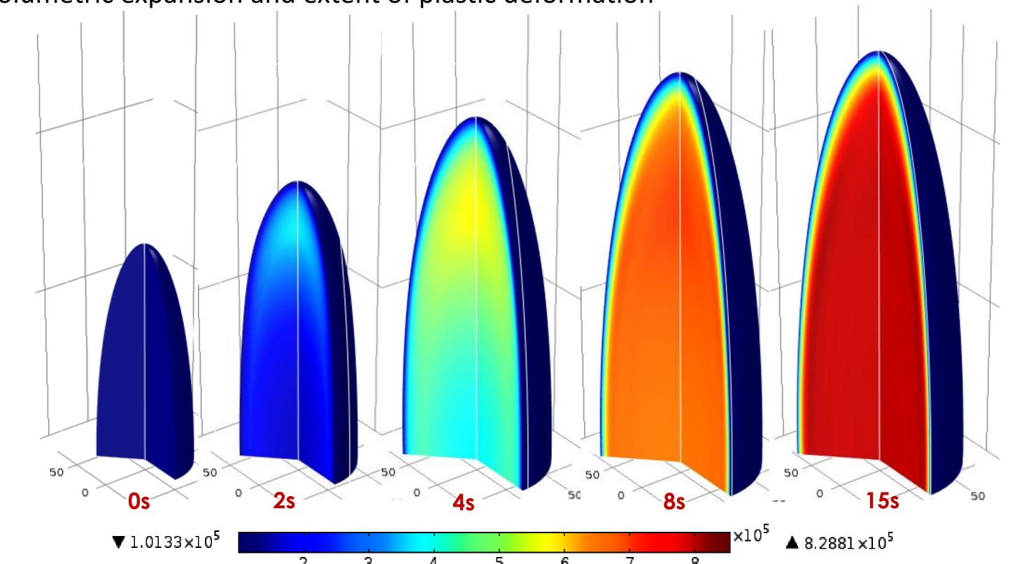
Simulated gas pressure generation with puffing time
