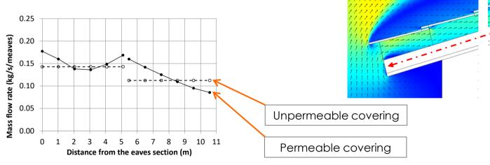
Results supported the submission of an EU project, aiming to improve the air permeability of vented tiled roofs, in order to reduce the building cooling demand in hot climates. (2014)
